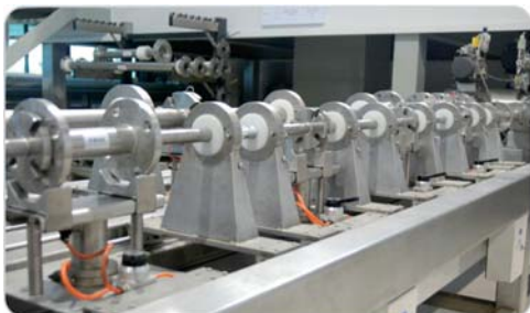
Piping system I (Max capacity for four meters calibration simultaneously in above system.)
